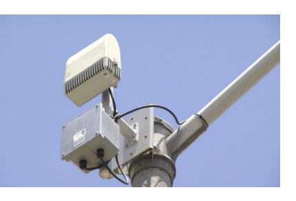
AGLS is a system designed to detect, record, and locate the sound of gunfire using sensitive microphones and sensors.
