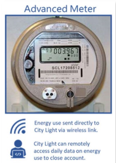
OCA infographic showing relevant features of SCL's advanced meters.
