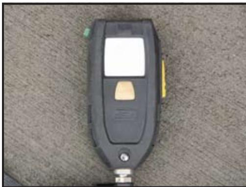
The ICM-Tx is an intrinsically safe, integrated heads-up display and an inline PASS (Personal Alert Safety System) device.
