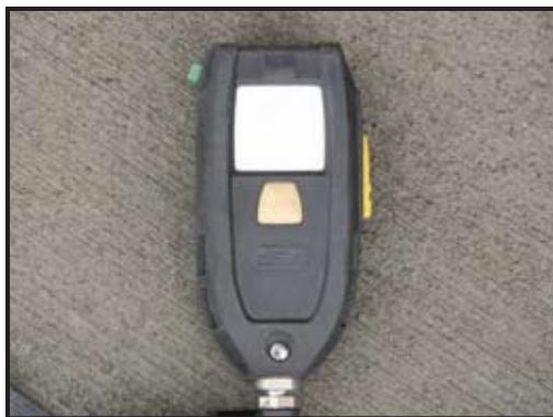
In the event that the user remains motionless for approximately **20** seconds, the ICM-Tx will enter into a pre-alarm mode. During the pre alarm mode, a RED light on ICM will flash and an audible signal will begin. Moving or shaking the ICM-Tx at this time will reset the ICM into normal operation and restart the **20** second countdown.
