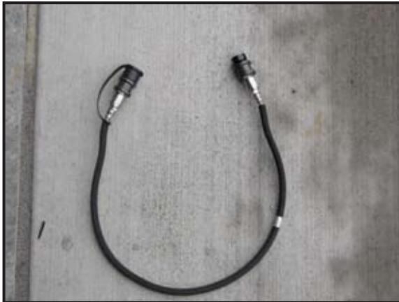
The Seattle Fire Department SCBA's are also equipped with a means to trans-fill another member should he/she become low on air while in a IDLH environment. A 3' high- pressure, emergency trans-fill braided hose (picture) capable of transferring air from a "donor" to a "receiver" is supplied in a kevlar pouch located on the left side of the waist strap. An emergency trans-fill should only take place in
