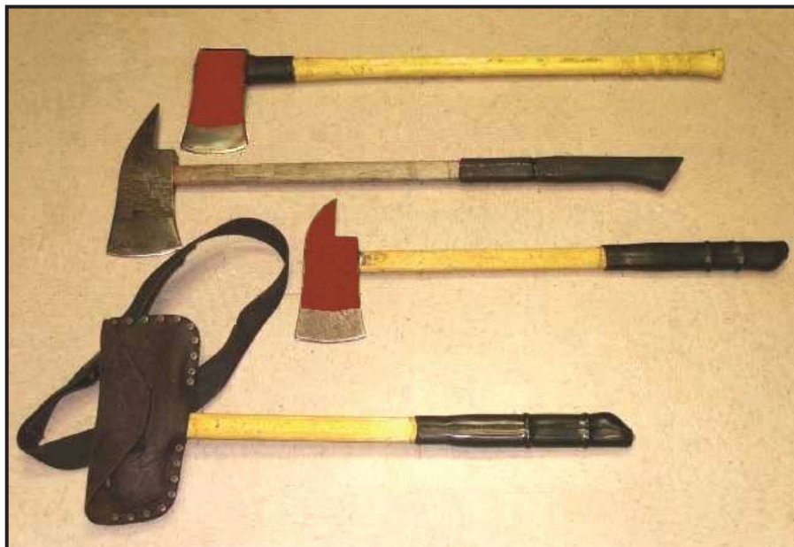
Top to bottom: HD Flat Head axe, HD Pick Head axe, Service axe, Service axe in belt scabbard
