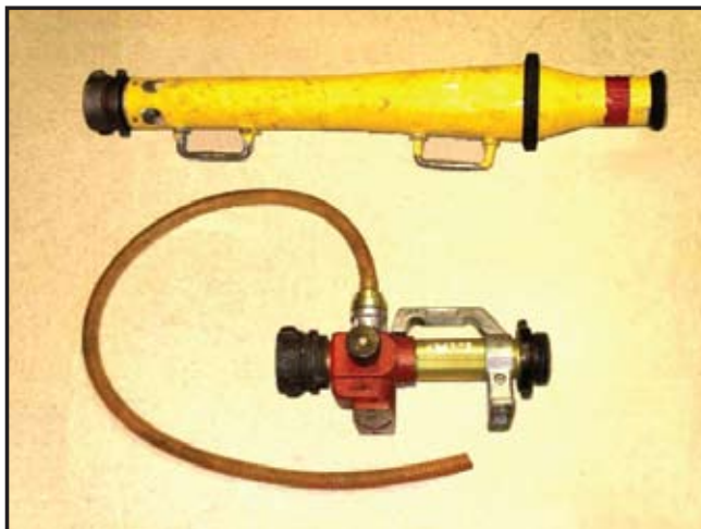
Low Expansion Foam Nozzle (top), 120 GPM Foam Eductor (bottom)
