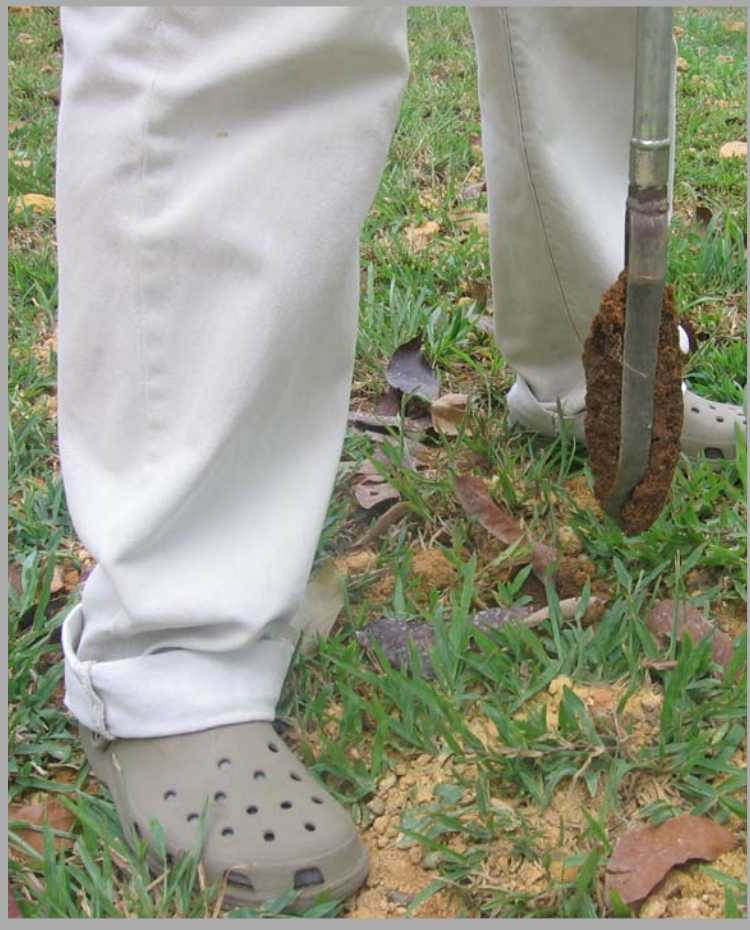
Examining a soil profile with a Dutch soil auger
