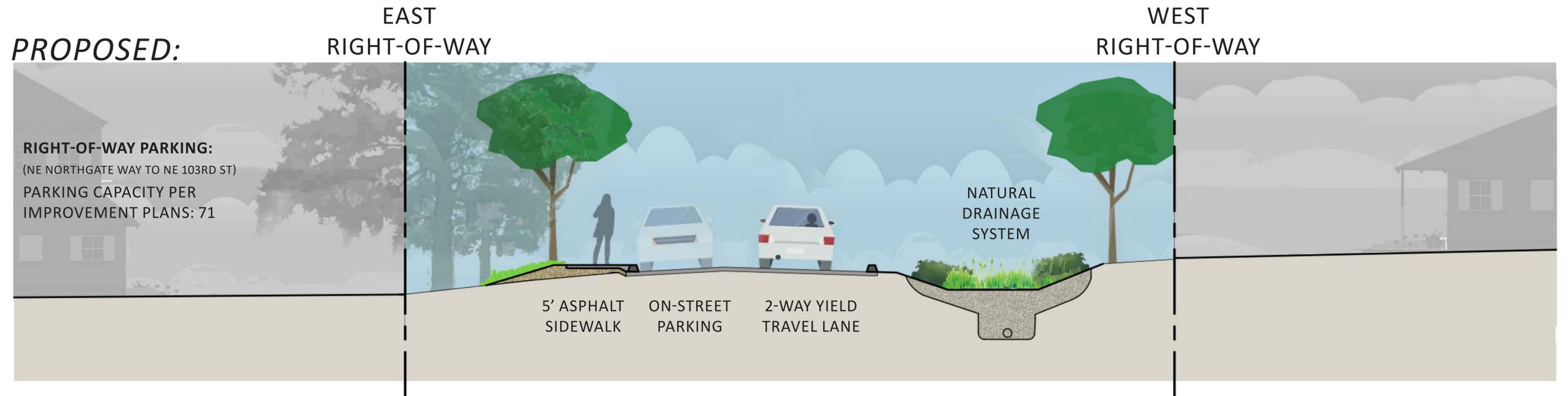
PROPOSED TYPICAL STREET SECTION WITH CURBING BOTH SIDES,
