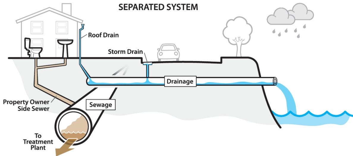
**Figure 3-3. Separated storm sewer system**
