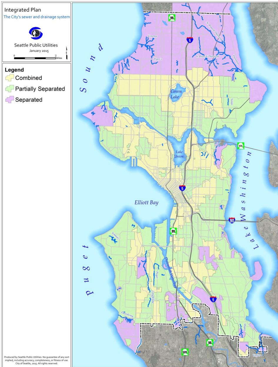
Figure 3-1. The City's sewer and drainage system
