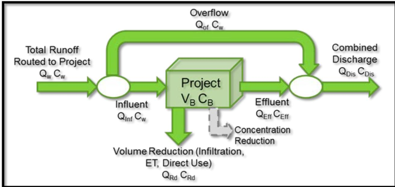
Figure 6-1. Flow chart used for stormwater project evaluation
