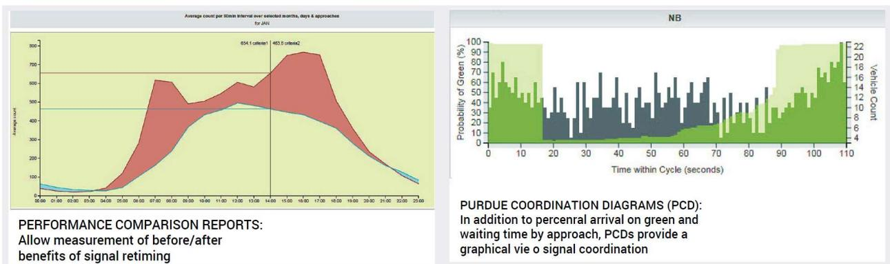
**Figure 10: ATSPMs Will Provide Analytics to Support the MICMA Evaluation and Ongoing Performance Monitoring**
