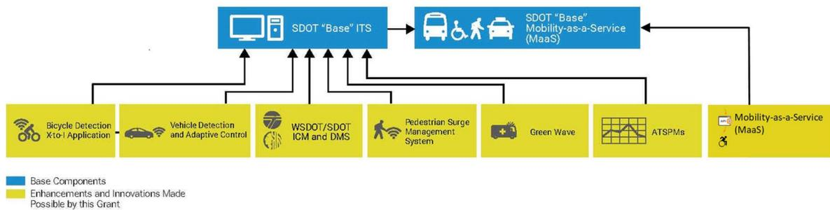
**Base ITS.** SDOT has programmed funds to install systems to address the major and unpredictable congestion in the UW subarea. Core systems to be installed as part of Base ITS include:
