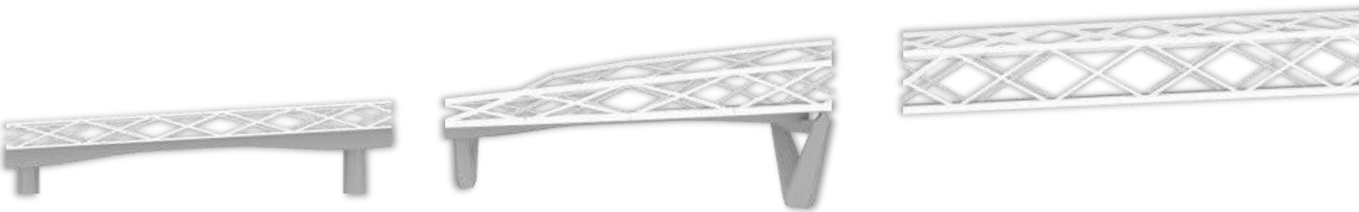
Concrete Girder ↔ Transitional Truss ↔ Structural Steel Tube
