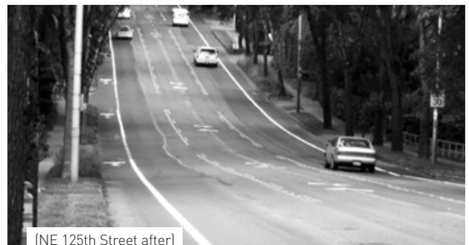
After changes were made to NE 125th Street to separate bicyclists and slow speeding cars, the collision rate for everybody went down 10% and the rate of collisions with injuries went down 17%.
