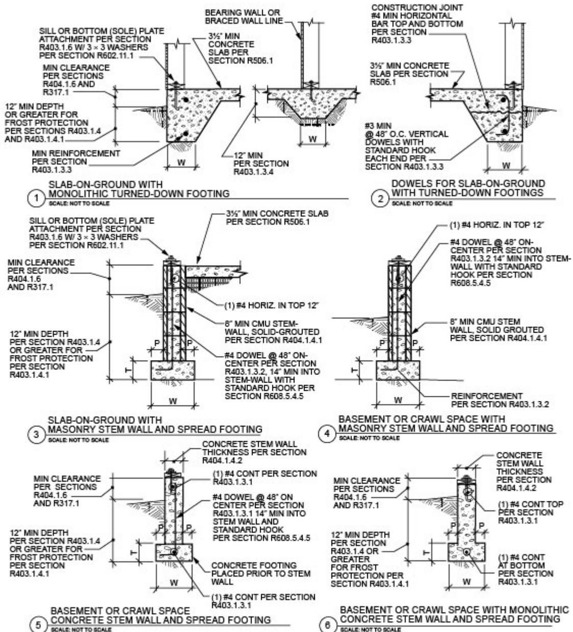
W = Width of footing, T = Thickness of footing and P = Projection per Section R403.1.1
