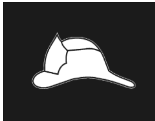
FIGURE 403.6.1.5.5 FIRE SERVICE ACCESS ELEVATOR SYMBOL
