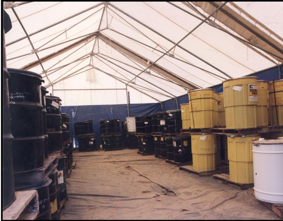
Figure 13. Covered and Secured Storage Area for Containers.
