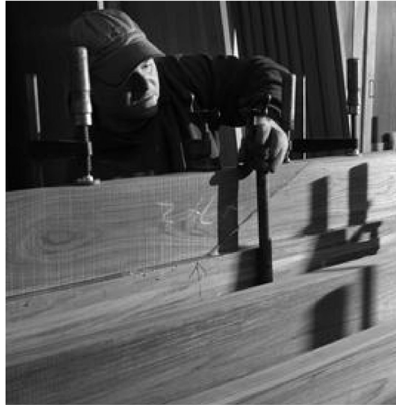
Jeff Krapf frame department woodworker at O.B. Williams Co., works on gluing and clamping a scarf joint of what will become a 25-foot-long, 2-inch-thick teak bar top. O.B. Williams Co., an architectural woodworking company, has been on First Avenue South in Sodo for more than 100 years.
