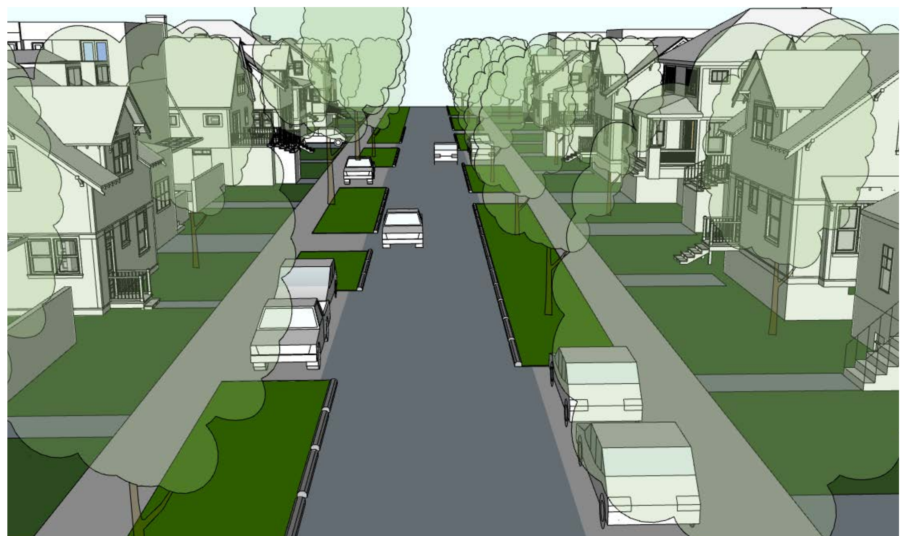
Larger planting strips may be more effective at solving drainage issues.
