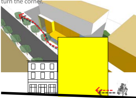
On sloping sites, set floor levels from the most visually prominent corner to avoid dead walls at the sidewalk level.
