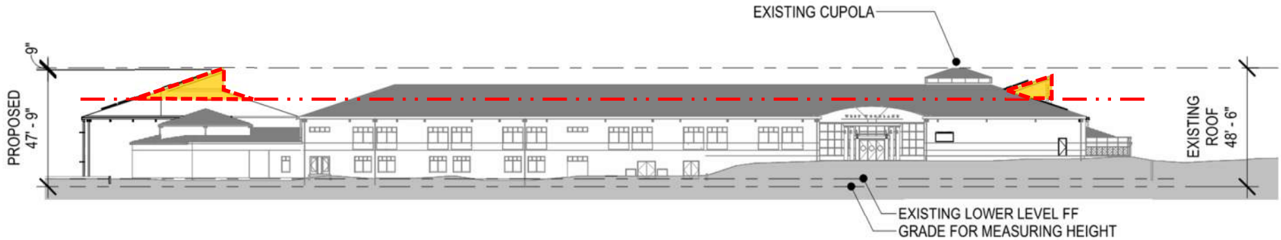
BUILDING HEIGHT - EAST ELEVATION
