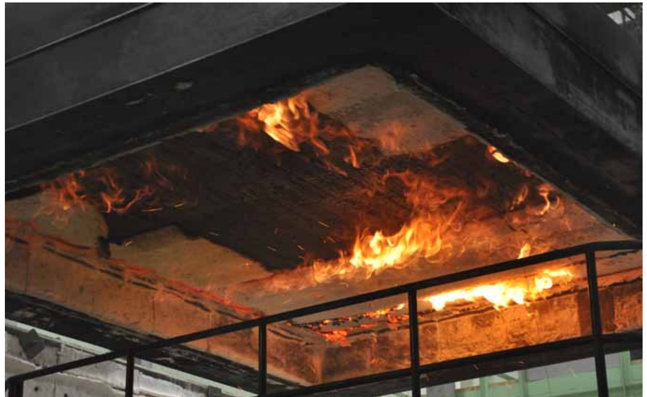
CLT floor fire testing. Source: FPInnovations
