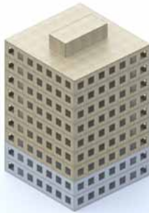
7-story CLT structure over a 2-story concrete podium
