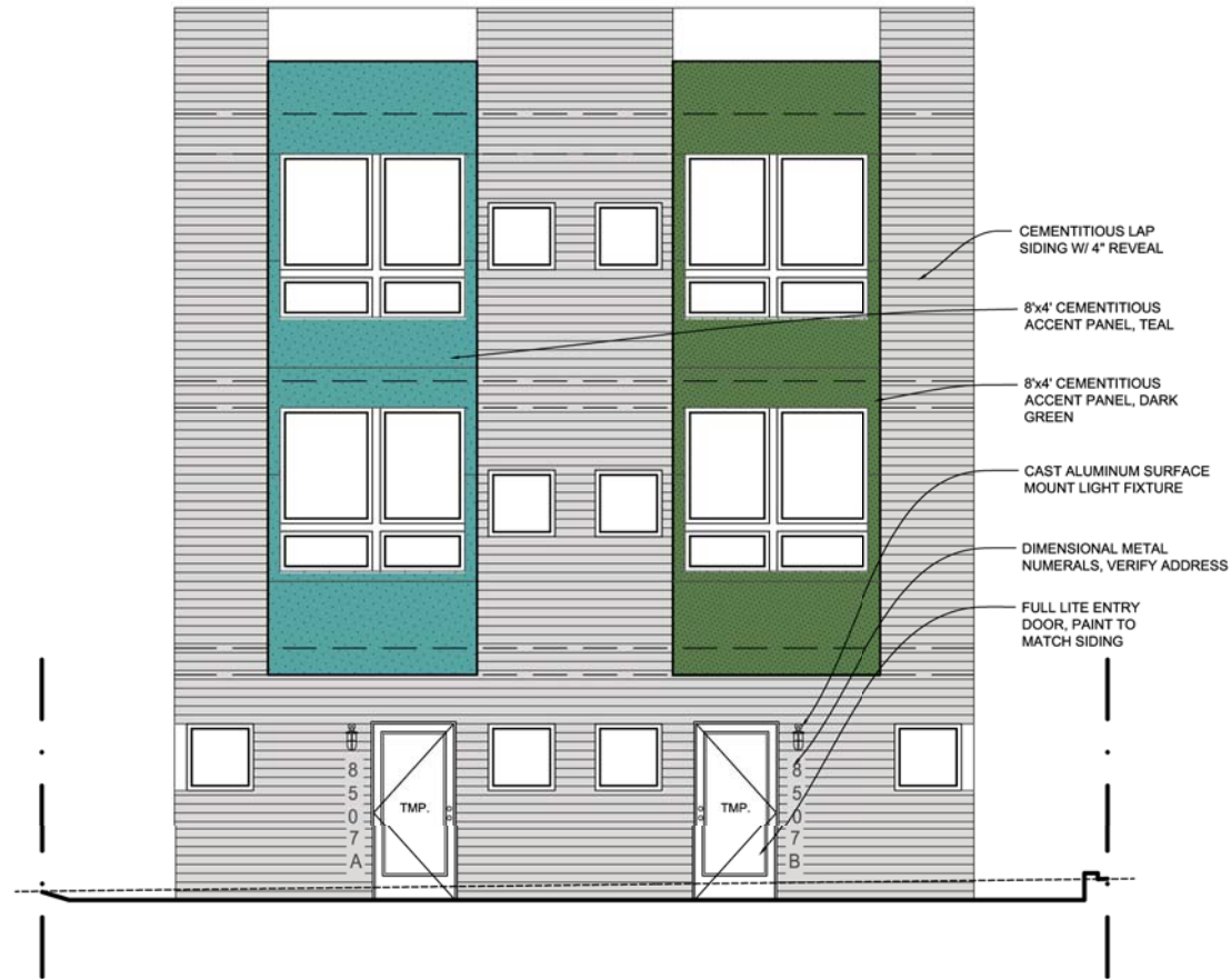
bldg B east elevation
