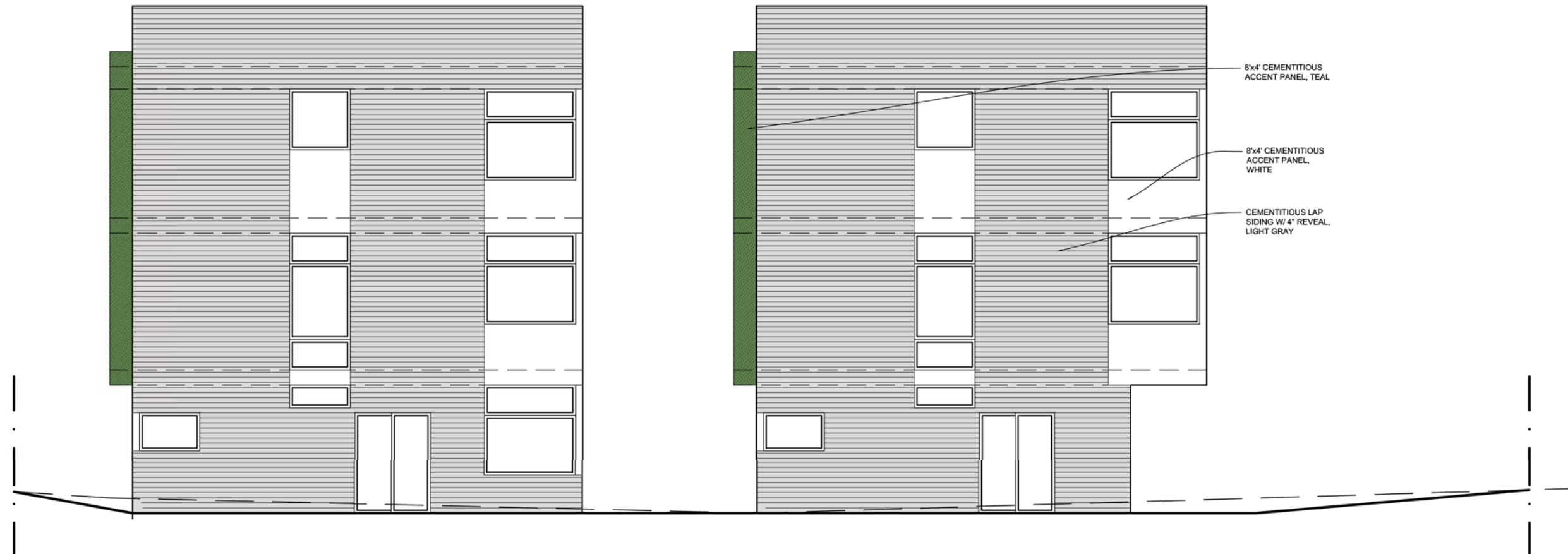
bldg A north elevation SCALE: 1/8" = 1' - 0"
