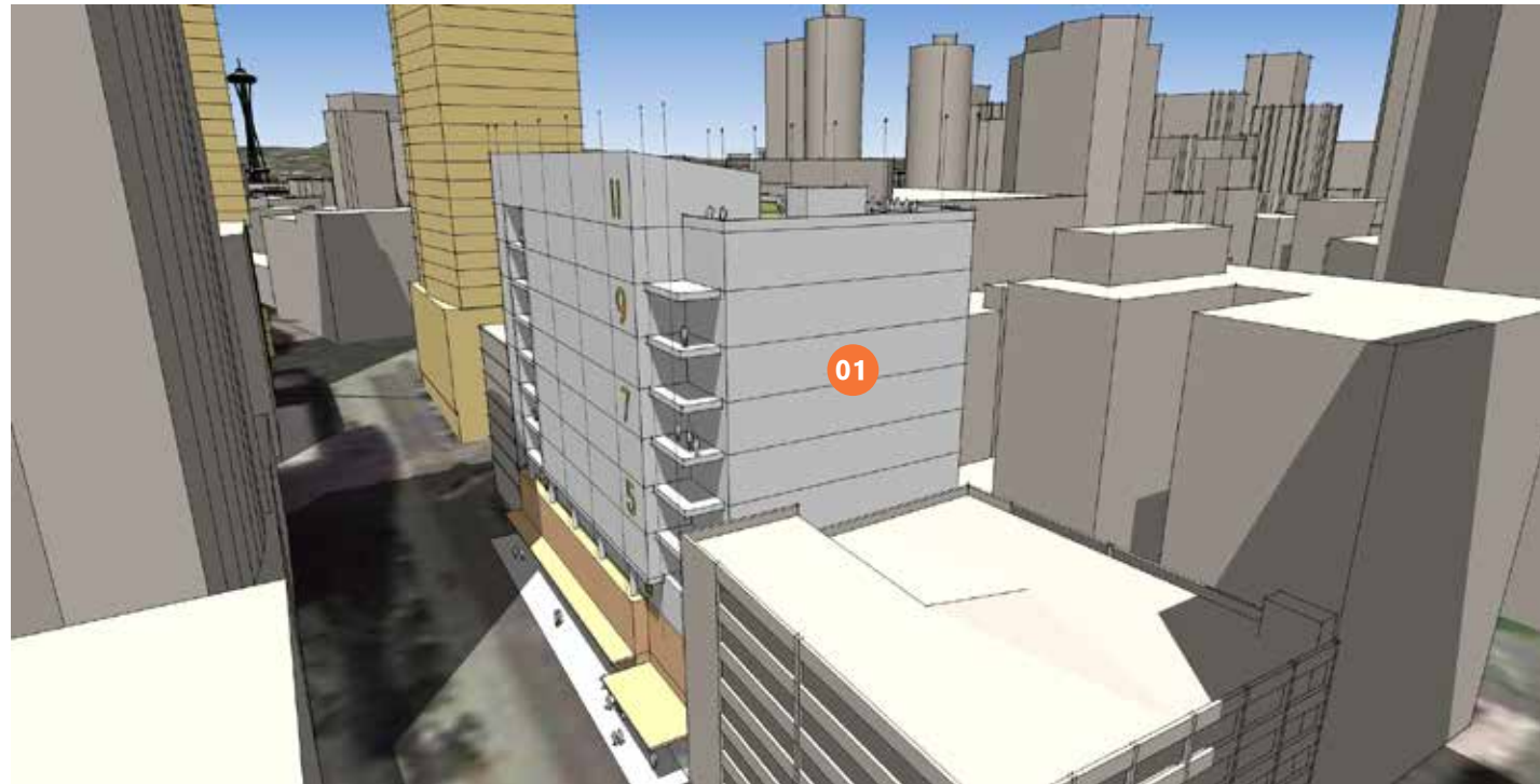
Two stacks of 25' x 12' outdoor rooms at West Facade. South party wall facade will be opaque. 01
