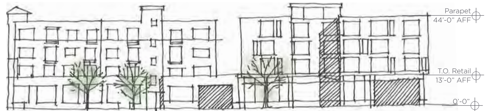
Proposed building facade aligns with key heights of adjacent building, but will provide more transparency at the retail level.
