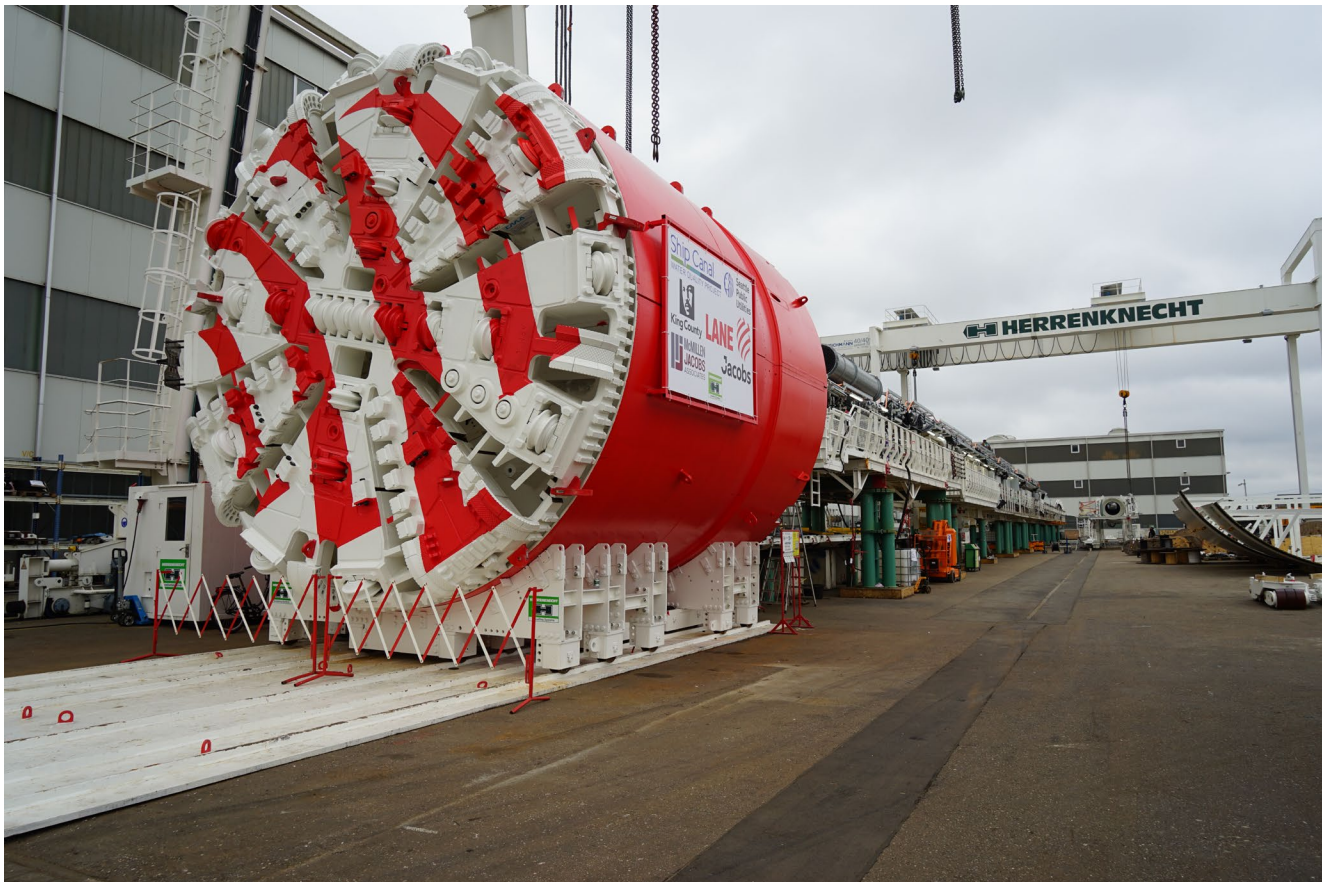
Figure 4-6. Completed Tunnel Boring Machine at Factory in Schwanau, Germany
