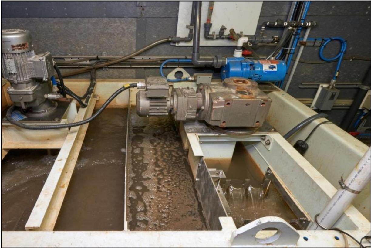
Figure 4-8. Pilot Test - Ballasted Flocculation Technology
