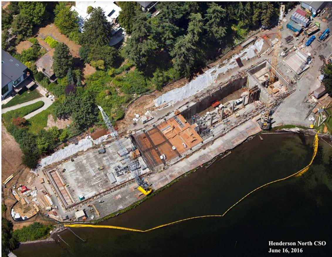
Figure 4-9. North Henderson CSO Storage Facility during Construction
