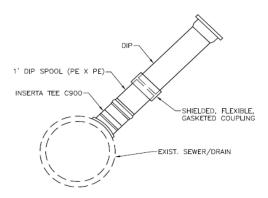
**Figure 3 Ductile Iron Lateral Connection**
