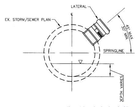
**Figure 1 Cross Section Standard Tee**
