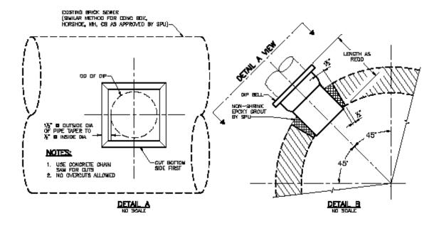
**Figure 5 Connecting to Brick Pipe**
