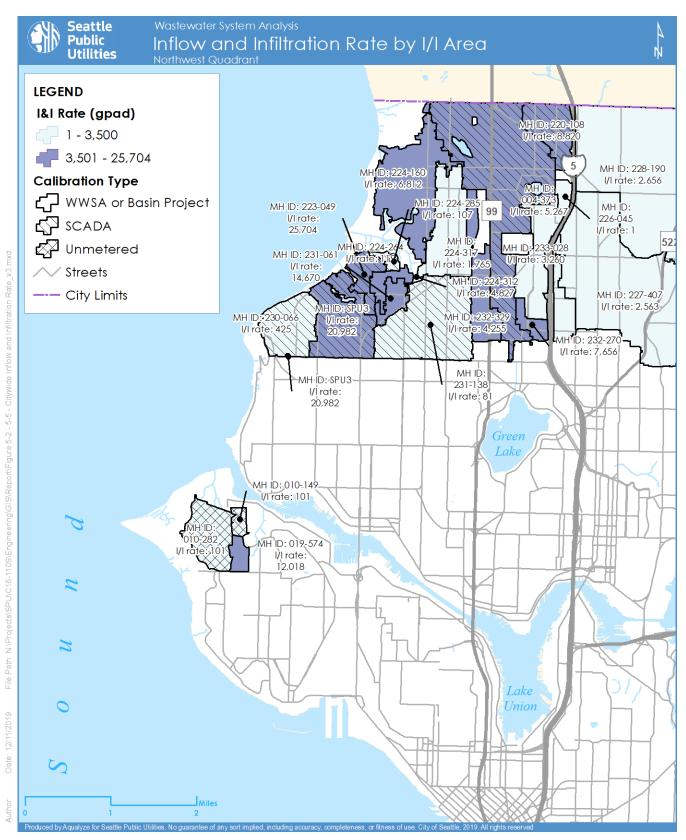
Figure 5-4. Inflow and Infiltration Rate by I/I Areas – Northwest Quadrant
