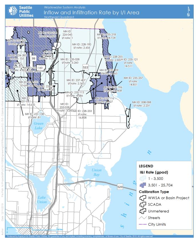
Figure 5-5. Inflow and Infiltration Rate by I/I Areas – Northeast Quadrant
