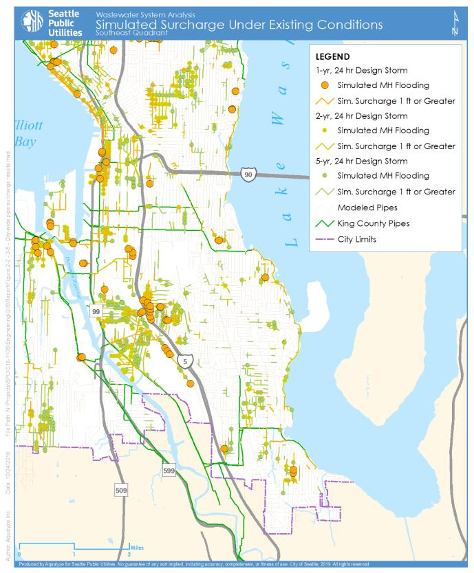
Figure 2-3. Simulated Surcharge Under Existing Conditions – Southeast Quadrant
