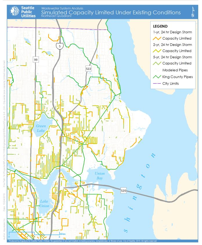
Figure 2-9. Simulated Capacity Limited Under Existing Conditions – Northeast Quadrant
