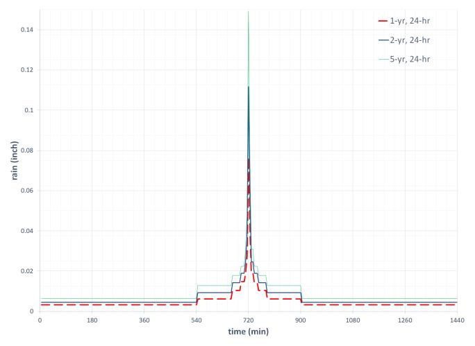
Figure 2-1. Synthetic Design Rainfall Hyetographs
