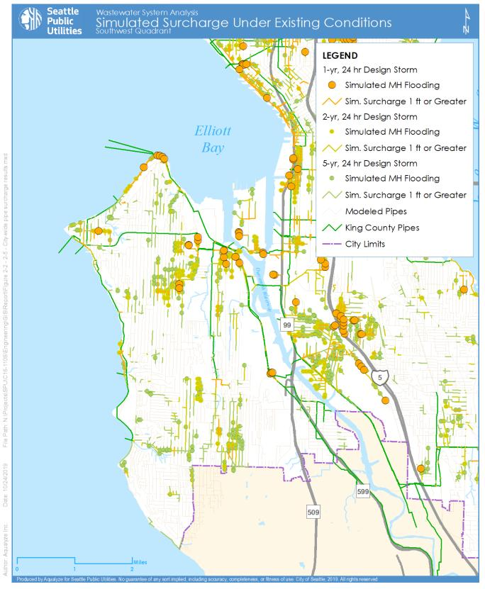
Figure 2-2. Simulated Surcharge Under Existing Conditions – Southwest Quadrant
