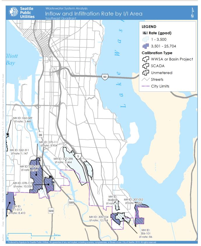
Figure 5-3 Inflow and Infiltration Rate by I/I Areas – Southeast Quadrant
