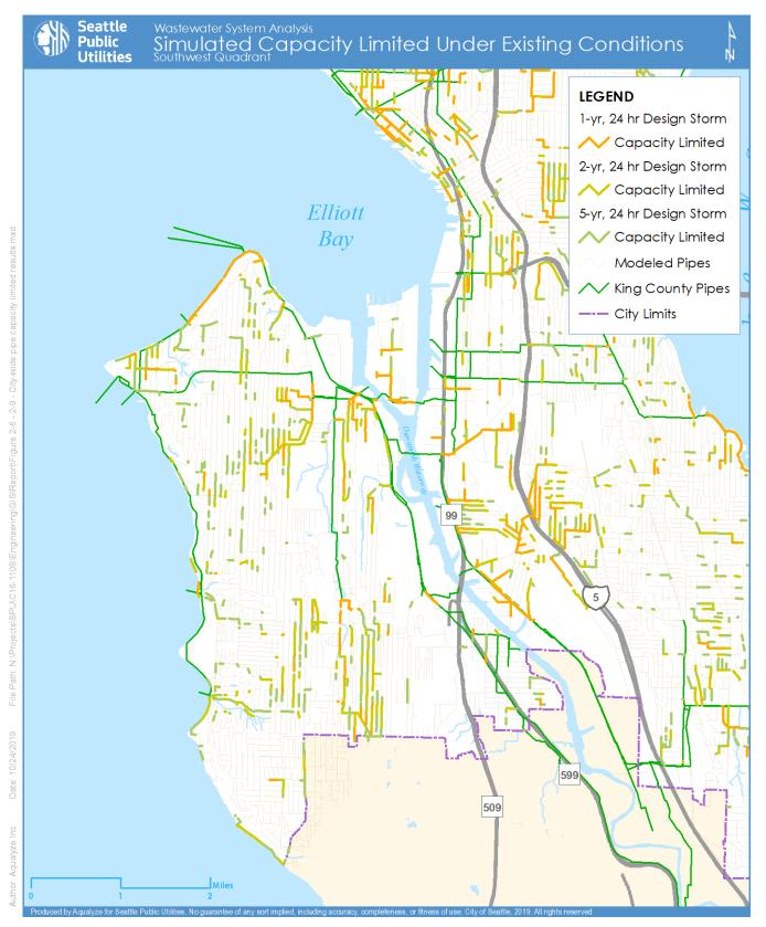
Figure 2-6. Simulated Capacity Limited Under Existing Conditions – Southwest Quadrant
