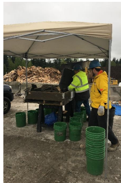
Sampling processing residuals at a mixed C&D recycling facility to confirm recovery of materials banned from disposal.
