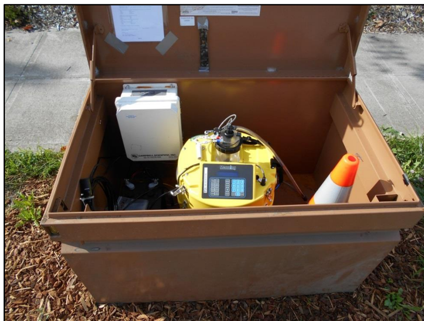
Figure 16. Cabinet containing sampler (yellow) and data logger enclosure (white)
