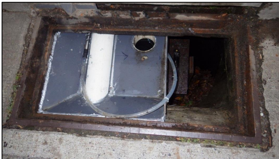
Figure 14. Sampling tray installed in inlet (inlet grate removed)
