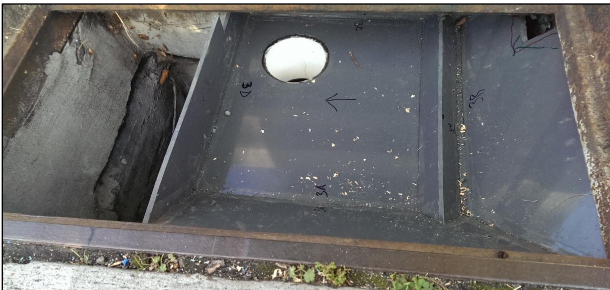
Figure A2. Sampling Tray Installed in Inlet (inlet grate removed).
