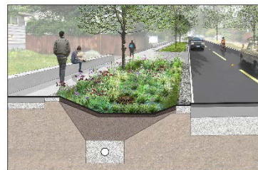
Figure 2. Sample of new sidewalk and natural drainage system
