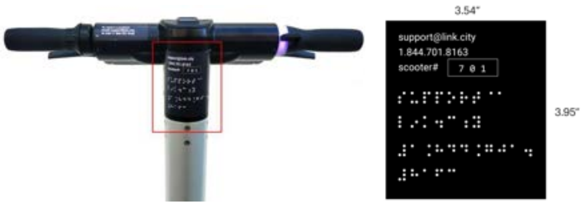
Braille identifier on the neck of each scooter with contact information for our support team (left) in ADA approved sizing (right).
