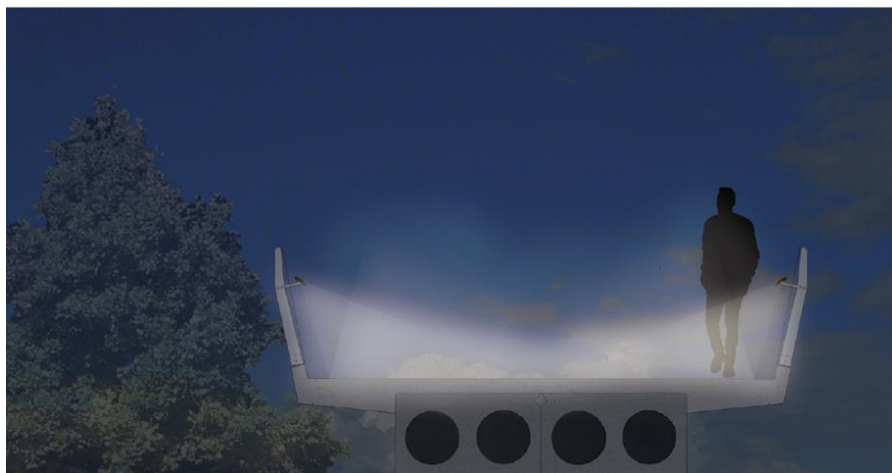
Typical handrail LED light fixture
