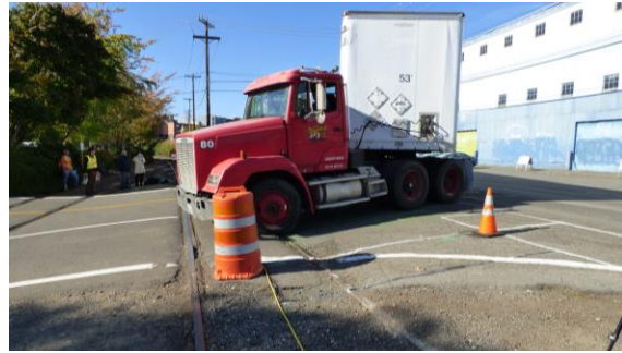
An alternate angle of the tractor-trailer completing a right-turn into the driveway. There is sufficient space in the driveway crossing for the truck to complete this maneuver.
