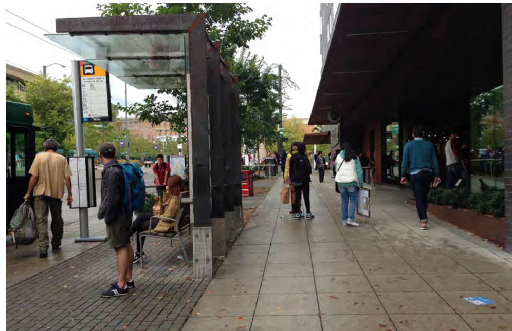
Concrete pavers are used to distinguish bus waiting areas on Campus Parkway in the U District.
