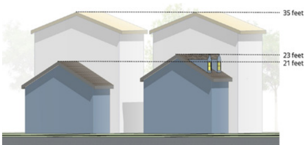
Exhibit 2-8 Illustration of Roof Features
