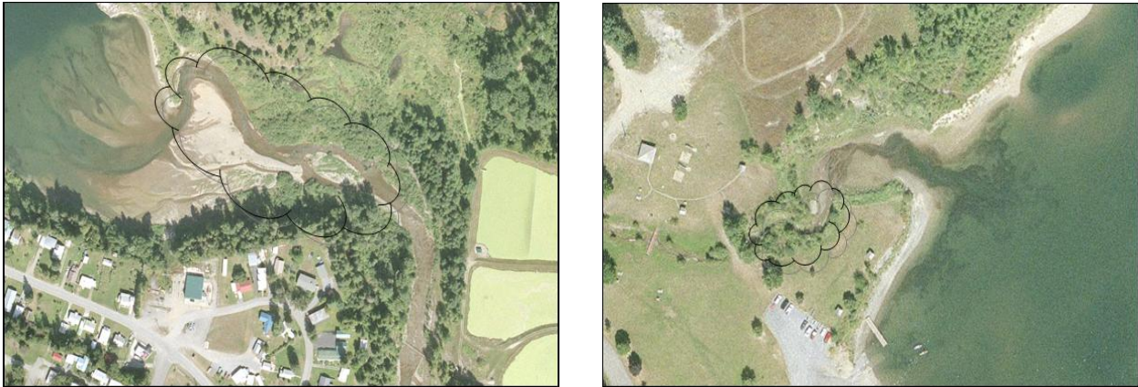
Figure 5.1-4. Possible areas for LWD placement in the upper deltas of Sullivan (left) and Linton (right) creeks.
