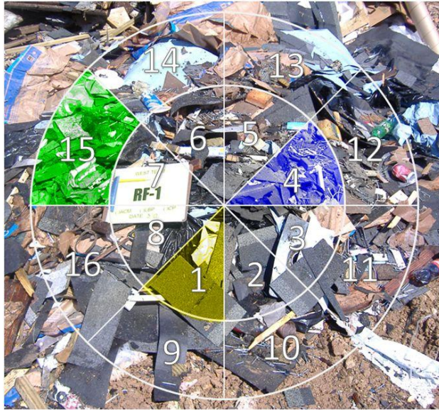
Figure 2. Visual overlay for Stockpile Method showing “cells” of material
