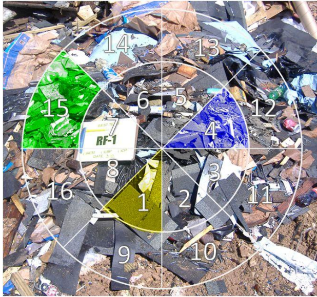
Figure 4. Visual overlay for Stockpile Method showing “cells” of materials
