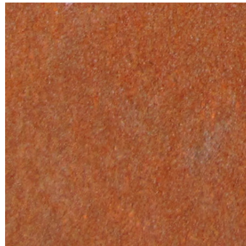
METAL ACCENT PANEL WEATHERING STEEL
