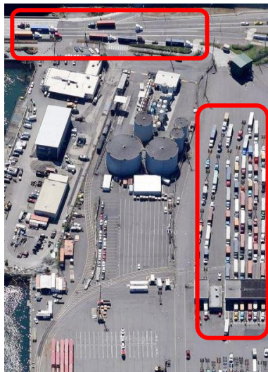
Figure 8. Gate 1 queue at ID gate (top) and transaction gates (bottom).
